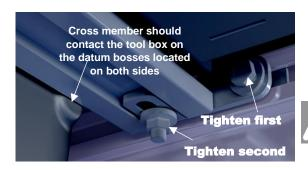
Tightening the striker nuts will firmly seat the cross member against the rear of the tool box.
