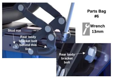
Install and hand tighten only, the stud nut on both sides of the truck.
