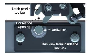
Closing the cover for the first time, check the relationship between latch pawl and the striker as the cover approaches the closed position. The top jaw of the horse shoe shaped opening in the latch pawl should be centered over the striker pin as it approaches the pin.
