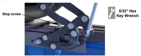
2. Remove the bedrail stabilizer bolts (1/side) – these parts are located at the end of the bed rails – reserve the parts for re-installation. <u>Not included with Tundra</u>.
