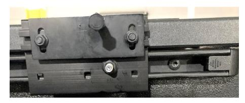
With the rear bedrails positioned approximately twelve inches from the tailgate, align the mounting stud with the rail mounting hole and loosely install the stud nuts.
