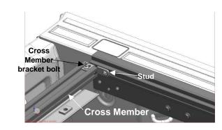
Parts Bag #4 Slide a single stud plate into the front end of the bedrail channel on both sides
