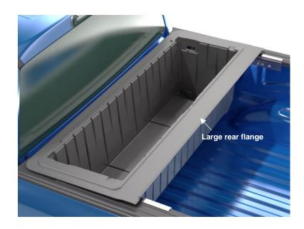
Load the tool box into the opening between the head board and the cross member. The large flange is positioned towards the rear of the truck.
