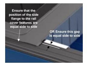
To locate the tool box in the correct position relative to the truck.
