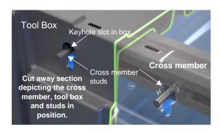
Lift the rear of the compartment upward to allow the cross member to be slid into the channel on the underside of the rear flange.
