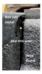
The truck bed itself is a source of water leaks into the bed. These pathways don't necessarily represent a threat to your gear but can generate a noticeable deposit of water on the floor of the box.
