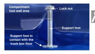
Loosen the lock nut and turn the support foot downward until it rests on the floor of the truck box. Retighten the lock nut to secure the support foot in place. The nut is located on the underside of the box for some applications
