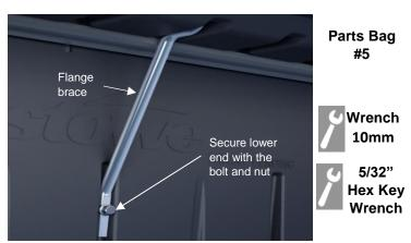
Install the tool box rear flange brace by inserting the top end of the brace into the underside of the flange and placing the lower end of the brace against the front face of the box.
