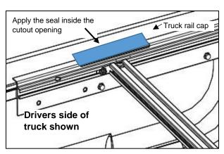
After installing the bed rails install the bed rail seals.
