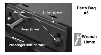
To install the striker spacer plate lift the cross member upward from underneath the tool box flange which will lift the two mounting studs. Insert the striker spacer through the round holes in the keyhole slot Load the front striker to the spacer and hand start the stud nuts.
