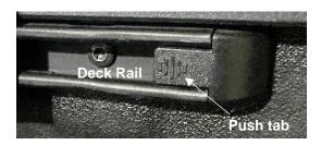
Remove the end caps from the tailgate end of the truck deck rails.
