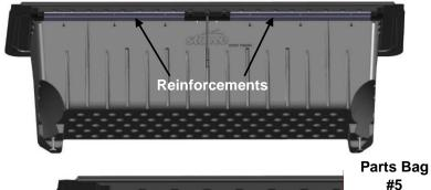
Install the six (6) attachments screws to secure the rear flange reinforcements to the underside of the tool box flange. The screws will thread into the mounting clips installed in the flange.
