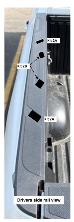
Clean the rib gaps with rubbing alcohol before applying the fillers in the locations shown below.
