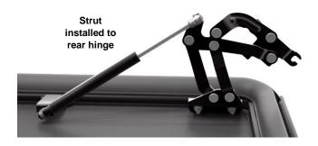
Install the rear struts by snapping the strut sockets over the ball studs on the hinge and cover.
