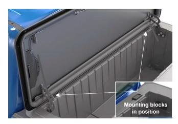
Place the front cover mounting Parts Bag blocks in the pockets on either side of the compartment front flange.
