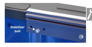
Wrench Remove the jam nut and thread the 10mm front stabilizer bolt through the bedrail until it firmly contacts the truck sheet metal but does not push the bed rail outwards.
