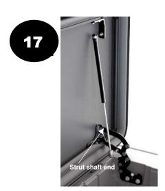
Install the struts by snapping the strut socket over the ball studs on the hinge and cover. Install the hinge end first.
