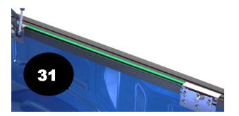
Measure from the rear edge of the front bed rail to locate the rear bed rail position.
