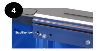
Loosen the jam nut and thread the front stabilizer bolt through the bedrail until it firmly contacts the truck sheet metal behind the bedrail.
