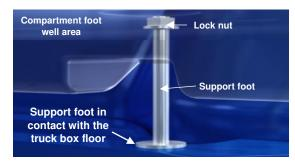
Loosen the lock nut and turn the support foot downward until it rests on the floor of the truck box. Retighten the lock nut to secure the support foot in place.
