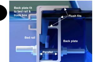
Raise the bed rail back plates <u>until flush</u> with the underside of the truck box while keeping it parallel to the back side of the bed rail.
