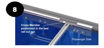
Loose assemble a nut to each stud.
