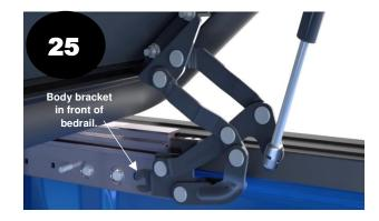
With the assistance of an associate lift the cover into position just behind the bed rails. Move the cover forward until the hinge body bracket starts to overlap the end of the bed rails.
