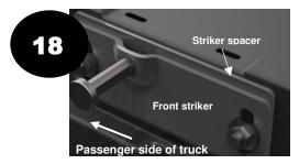
Install the front striker spacer through the rear of the compartment over the exposed cross member studs. Load the front striker to the spacer and hand start the stud nuts.
